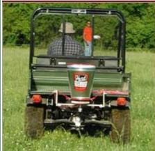
Applying fire ant bait using a herd seeder mounted on an ATV.
