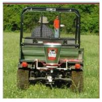
Figure 2. Applying fire ant bait using a herd seeder mounted on an ATV
